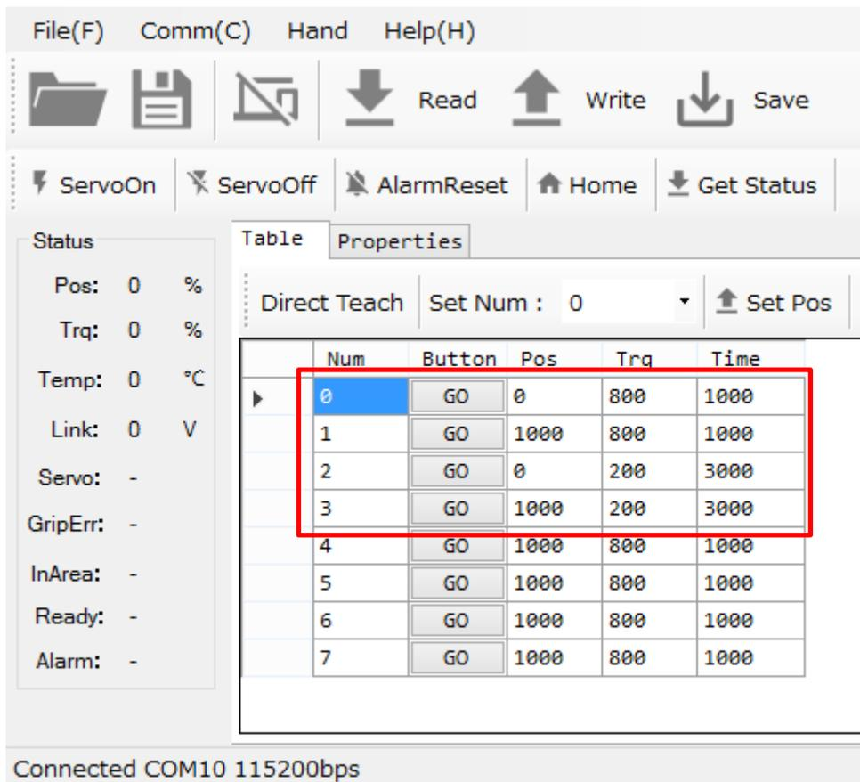
**Table 1 Example of robotic gripper operation parameter setting**
