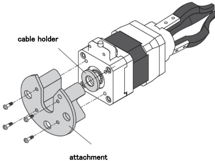
1. Attach the dedicated attachment to the robotic gripper body (A screw is included in the exclusive attachment.).
