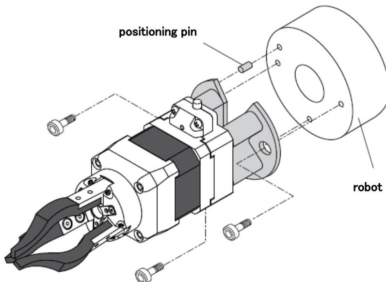
2. Attach the attachment to the robot end effector mounting surface.
